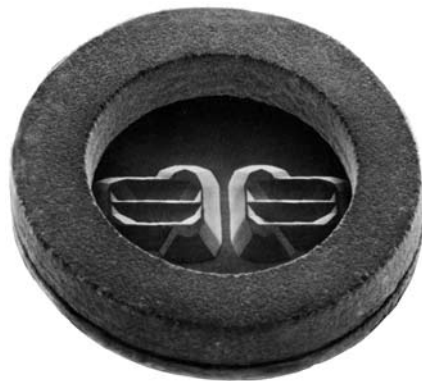
Figure 1 — Photograph of diaphragm taken with scanning electron microscope 0.05 in. (1.25 mm) O.D.
