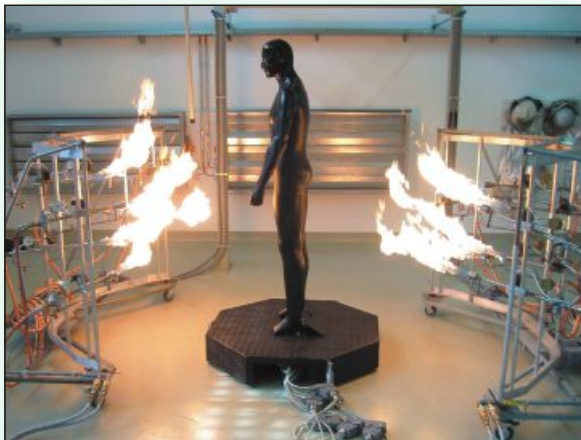
Testing of fire-resistant clothing by means of a dummy equipped with a great number of thermo-couples
