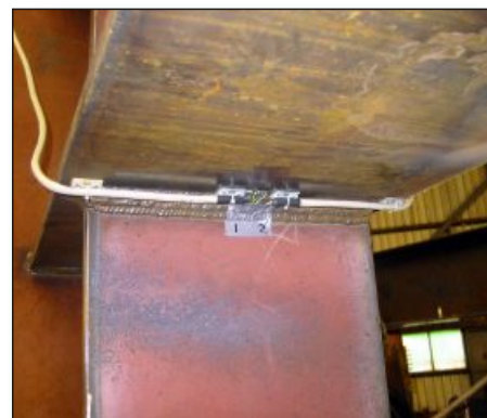
Testing for the maximum load in welded joints
