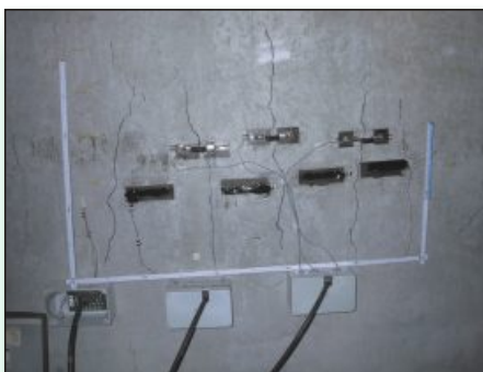
Monitoring cracks in concrete structures
